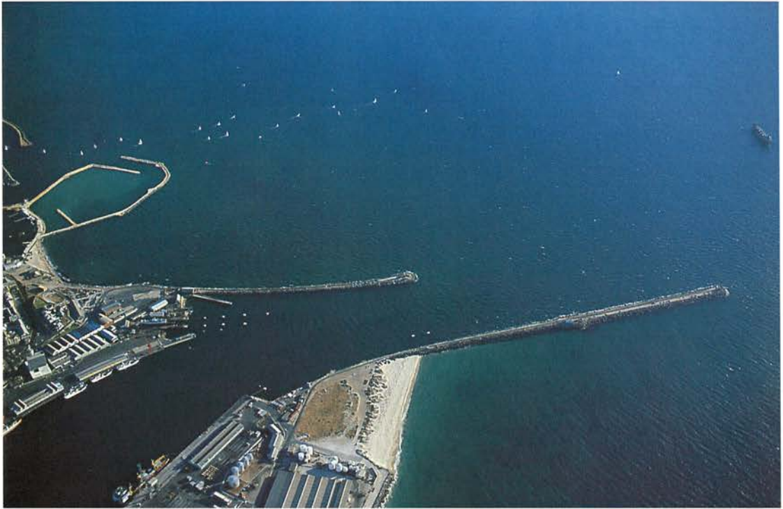
Port of Fremantle at the mouth of the Swan River. In 1892 moles were constructed to improve the entrance to the harbour. Photograph by Kevin Diletti.
